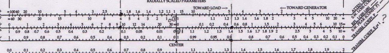
SWR = 2, RTN LOSS = 9.5 dB,  $P = 0.333$ , REFL. LOSS = 0.51 dB, 89% PWR FWD,
