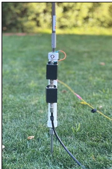
The Challenger+ backpack version is so compact and works so well, I am now using it at picnic table activations, too. As long as the feedpoint is at least 12" off the ground, it performs well in the field.
