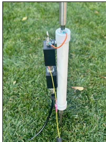
The Palomar™ 4:1 unun is mounted to the PVC tube with a small spacer and includes a 6" orange whip pigtail to a 3/8"-24 coupler nut on the top cap. The Palomar™ choke attaches securely to the unun with a PL-259 barrel connector.
