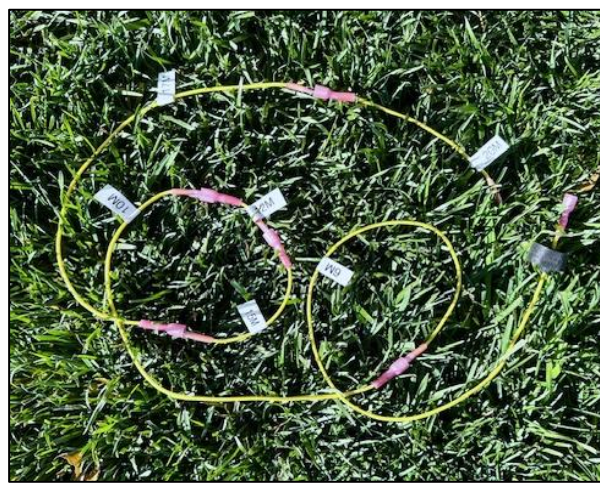
Each counterpoise segment is clearly labeled with a Brother™ label maker folded over on itself.
