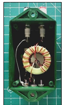
Low Insertion Loss with a 4:1 Unun
