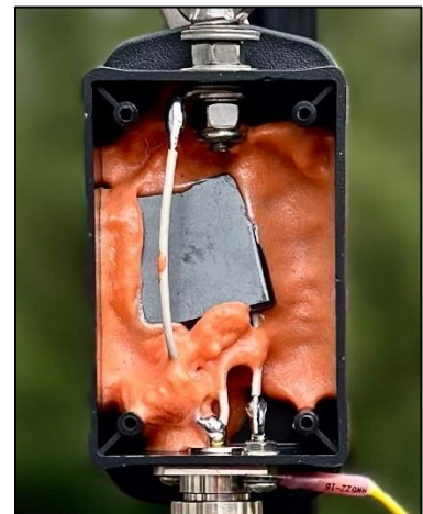
Palomar™ 4:1 unun uses a dual port 1 ¼" square ferrite bead.
