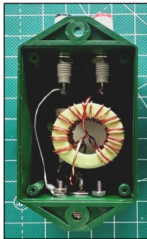
LDG™ 4:1 unun uses a ½" thick FT-140-43 toroid.
