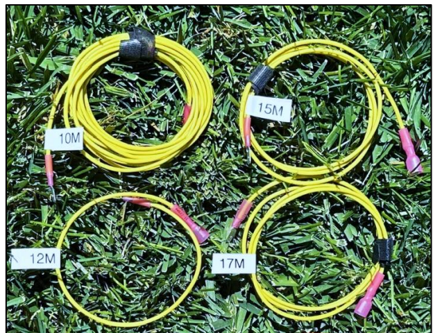
Each counterpoise segment is clearly labeled with a Brother™ label maker folded over on itself.
