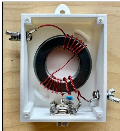
TennTennas™ 49:1 transformer uses a ½" thick FT-240-43 toroid.
