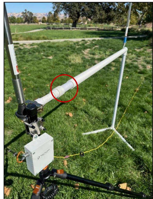
2 PVC tubes slide like a trombone to allow variable spacing between the elements
