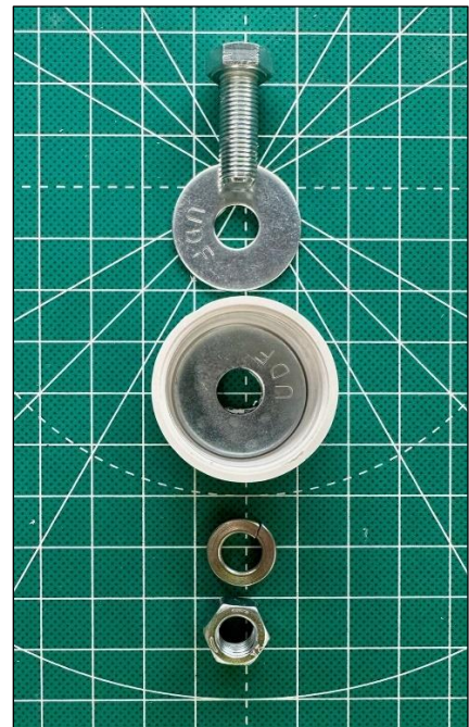
Drill a 3/8" hole in the center of end cap. Use 3/8"-24 hardware including 2 fender washers on both sides of the PVC end cap.
