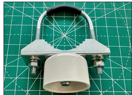
Before attachment, add 1/2" diam. shrink tubing on the U-bolt.
