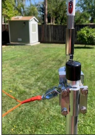
A **Chameleon™** 17' whip on a mirror mount is attached securely to a 2' aluminum tube with 1" OD. A **Mueller™** clip is used to combine two elevated tuned radials and clipped firmly to the mount to provide an effective elevated counterpoise.
