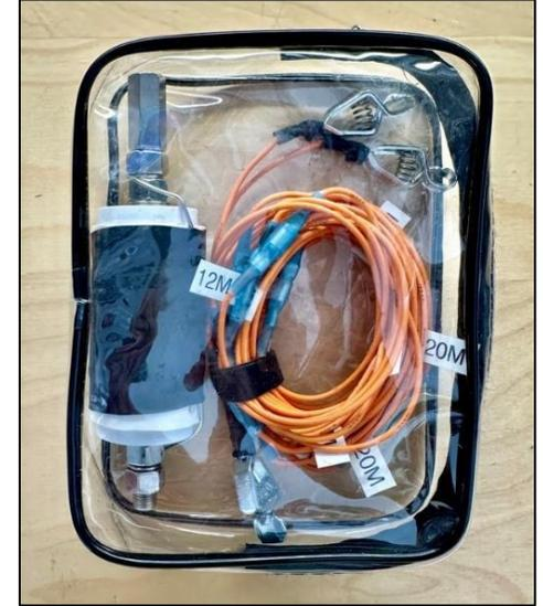
A **zippered clear plastic bag** (commonly used for travel toiletries) provides the perfect enclosure for the radial system and accessories. It also holds the **WRC™ Sporty Forty** for 40M operation and a **RigExpert™ Stick** analyzer for easy antenna tuning resonance in the field.
