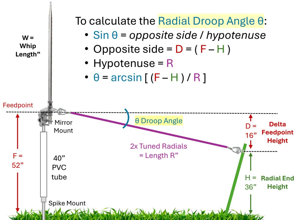
If you move the end stakes for each band change, your radial droop angle will change. Alternatively, if you insert a non-conductive segment in the line, the droop angle will remain consistent at the 20M band droop.
