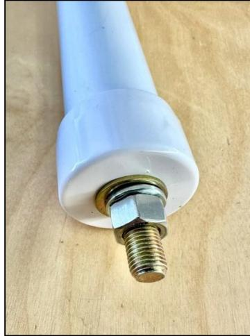
A 3/8" hole is drilled into the **PVC bottom cap** to insert a 3/8"x 24 bolt (1.5"- 2" long) and nut to easily screw into the **Chameleon™** spike mount or short tripod, e.g. WRC Mini-Pod.
