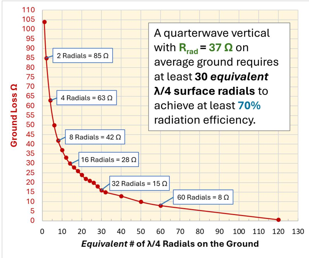
**Loss Resistance** = *Measured Feedpoint Resistance* - *Calculated Radiation Resistance*
