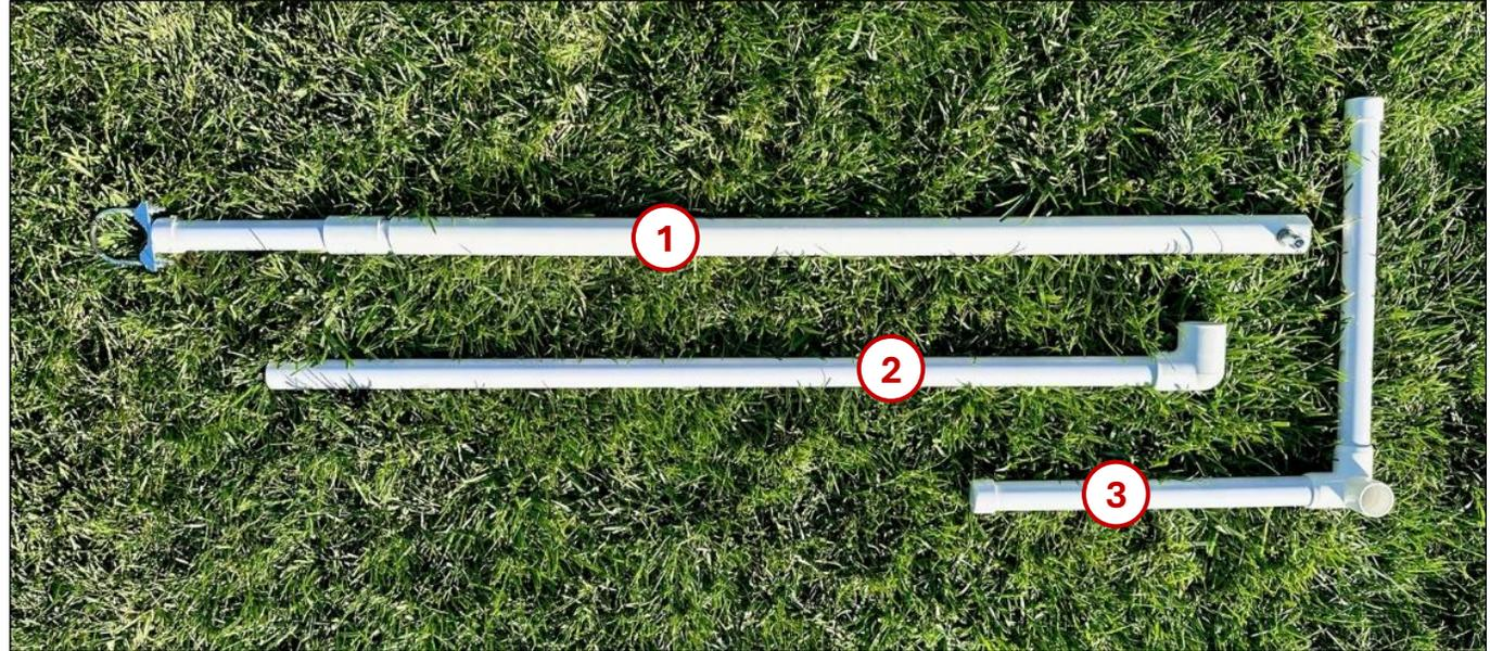
**Dominator Halfwave Beam Parasitic Director PVC Add-On** easily comes apart into three sections for **flat transport** and **fast deployment**:
