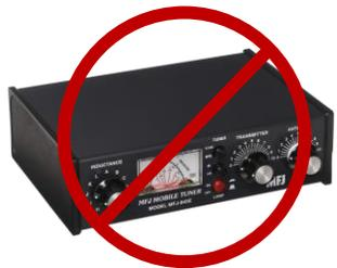
No tuner is recommended if SWR is less than or equal to 1.50:1 which implies 96% power transmitted
