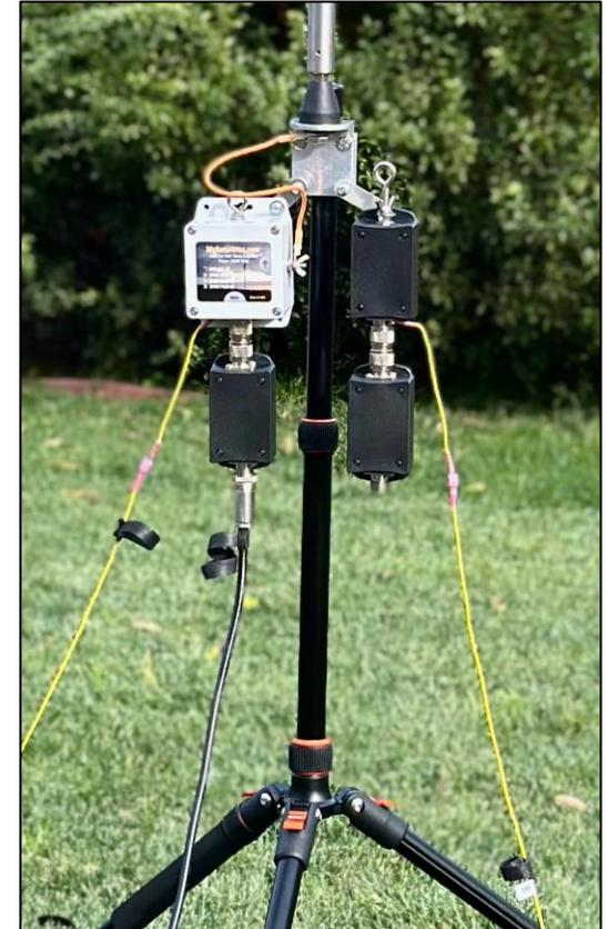
Dominator+ and Challenger+ mounted side-by-side on the Polarduck™ tripod.
