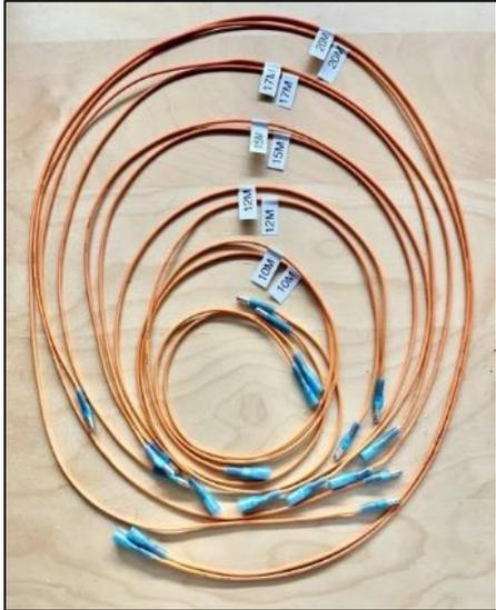
The **elevated radial system** is composed of pre-cut 18-gauge wire segments that are linked together within a string by spade connectors. These connectors allow the fast and easy insertion of a non-conductive segment to terminate the radial at that point for each band.
