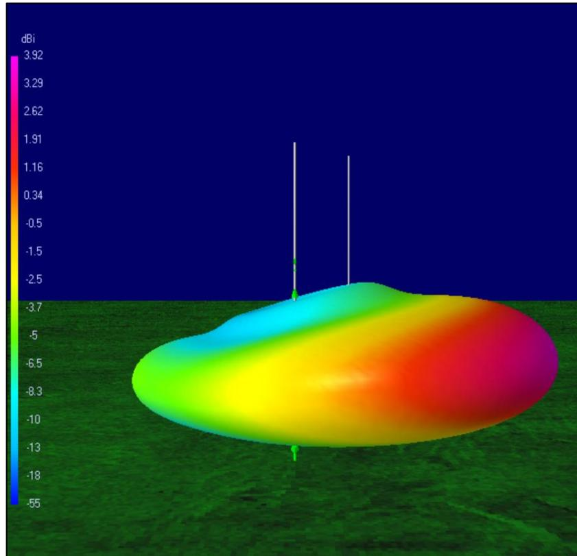
Purple and red edges of the radiation pattern highlight the strongest forward gain of the antenna 16 degrees off the horizon on 10M.
