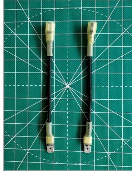
Two 4” **non-conductive radial segments** (using paracord) have spade connectors on each end. The segments are inserted in each elevated radial line to terminate it at the band of operation. By doing so, the fiberglass end stakes *do not* have to be moved for each band change.
