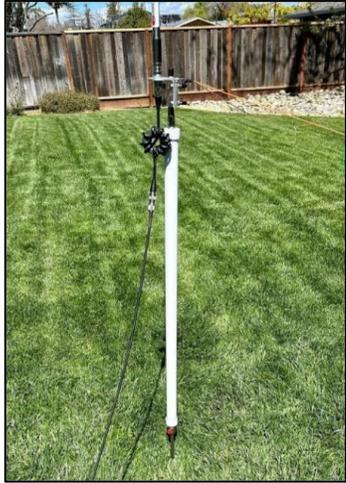
**PERformer** shown with a 40" furniture grade PVC tube (1" ID) on a **Chameleon™** spike mount. The non-conductive support structure provides both elevation and a secure mount for the telescoping whip and 2 elevated tuned radials.
