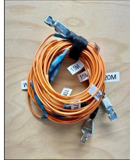
**PERformer elevated radial system** shown coiled up with a Velcro™ strap for easy transport and fast deployment. A **Mueller™ clip** is used at one end to combine the radials, and another at the end of each radial. Each band segment is clearly labeled.
