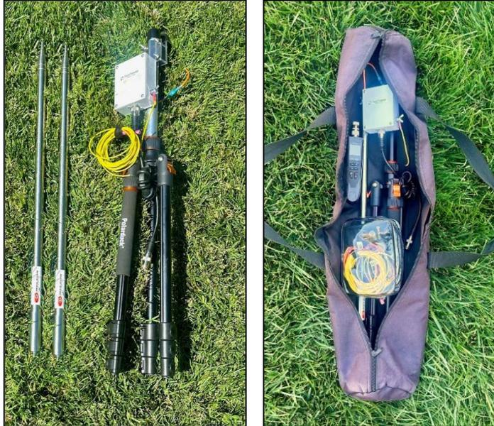
**Dominator Halfwave Beam** on a **Polarduck™ tripod** easily fits within a zippered **36” long photography bag** including both 25’ (or 17’) whips.
