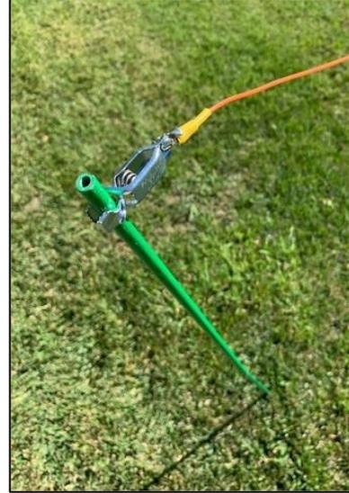
A **Mueller™** clip is used at the end of each elevated radial to attach onto a 48" fiberglass (non-conductive) stake. The clip can easily be slid up and down (droop) to finetune the feedpoint impedance for low SWR. These stakes are used for both deployment options.
