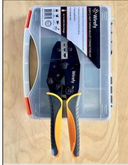
The ratcheting **Wirefy™ crimping tool** and heat shrink male/female **spade connectors** are used for fast and easy attachment of radial segments. The connectors not only have heat shrink tubing but also have internal glue that, when heated, provides a very secure connection.
