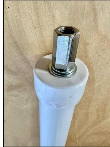
A 3/8" hole is drilled into the **PVC top cap** to insert a 3/8"x 24 bolt and nut (about 1.5" long) to accept a mirror mount that supports the 17' **Chameleon™** whip. A split lock and fender washer is used on both the inside and outside for a secure fit.
