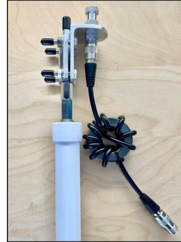
The mirror mount screws into the long bolt at the PVC top cap for the telescoping whip. A **Palomar Engineers™** RF choke (or suitable equivalent) must *always* be used at the feedpoint to isolate the coax shield from the antenna system.
